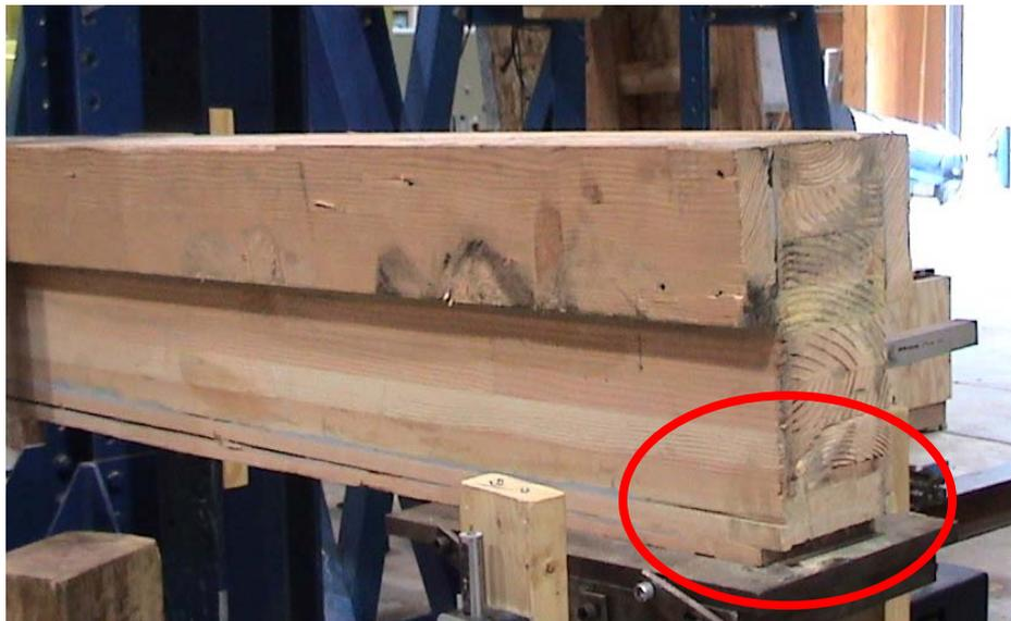
**Figure 15:** R-5 horizontal shear failure between the steel reinforcement and the wood directly above it from the load head to the right beam support. Note bottom half of reinforcement lamination pulled toward load head.
