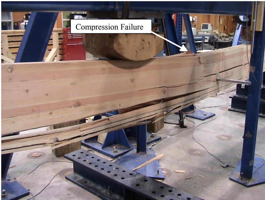
**Figure 12:** Hardwire Reinforced Beam R-4 - Note Compression Failure on the Wood
