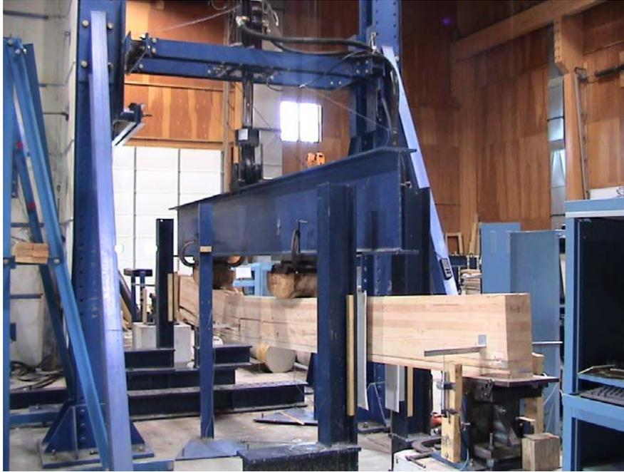
**Figure 2:** ASTM D 198 Four-Point Bending Test Set up
