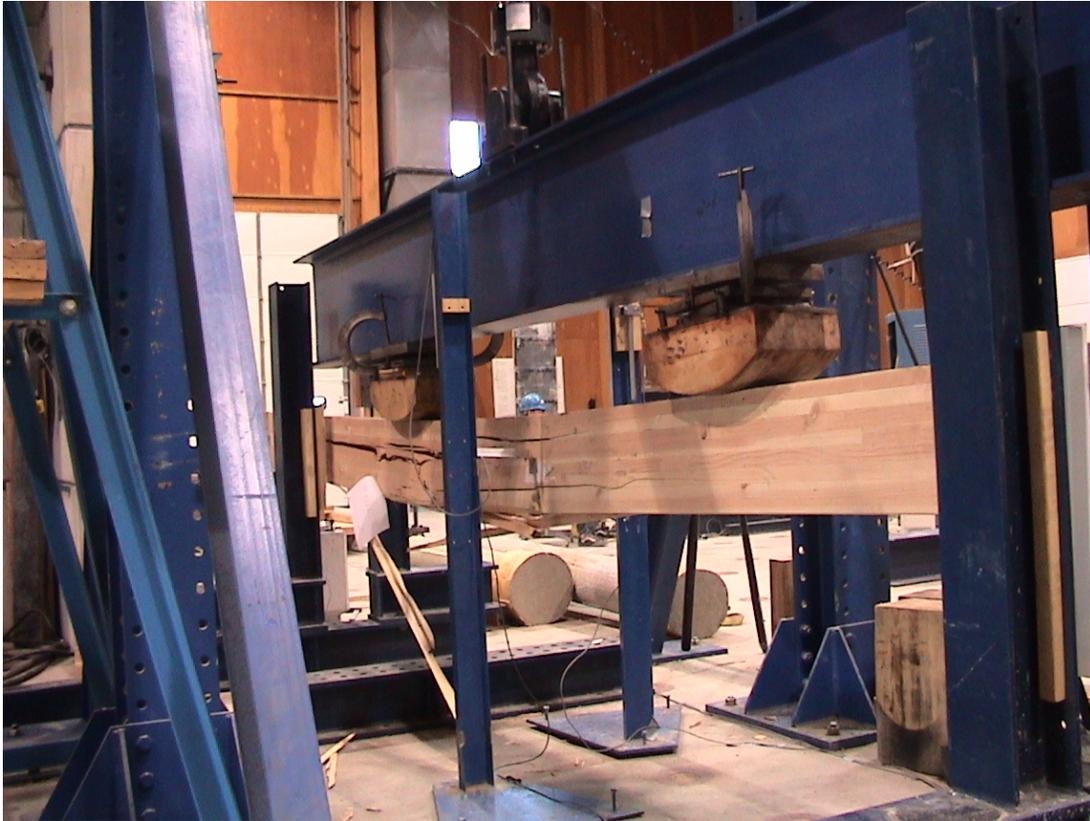
**Figure 6:** Control Beam Failure: 24F V4 DF/DF, no Reinforcement
