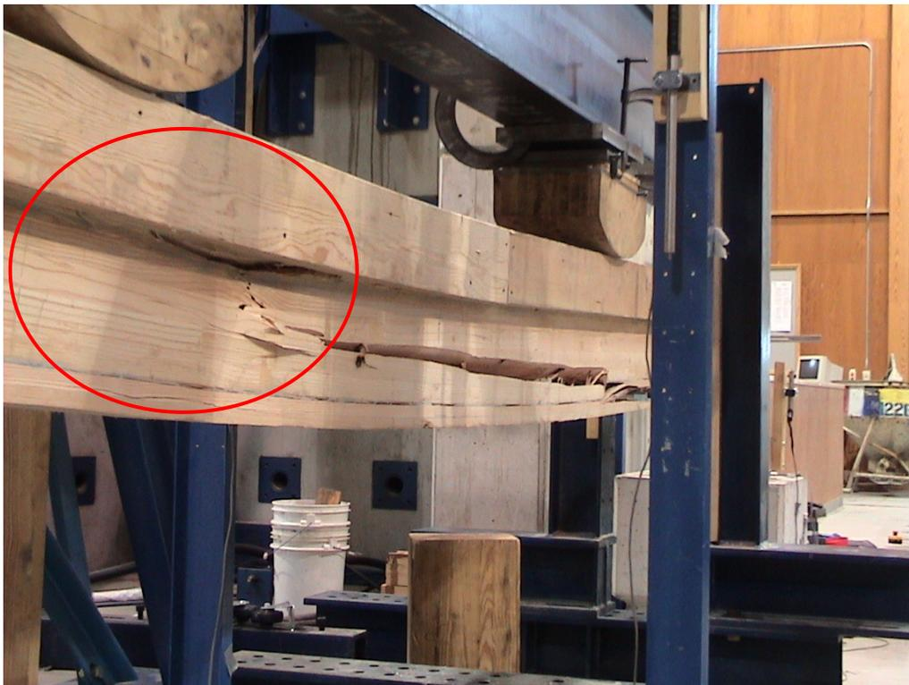
**Figure 13:** R-5 Failure: Possibly starts as horizontal shear failure under the left load head
