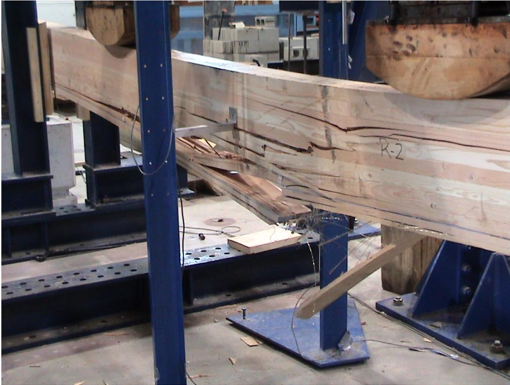
**Figure 8:** Hardwire Reinforced Beam R-2 Tension Failure
