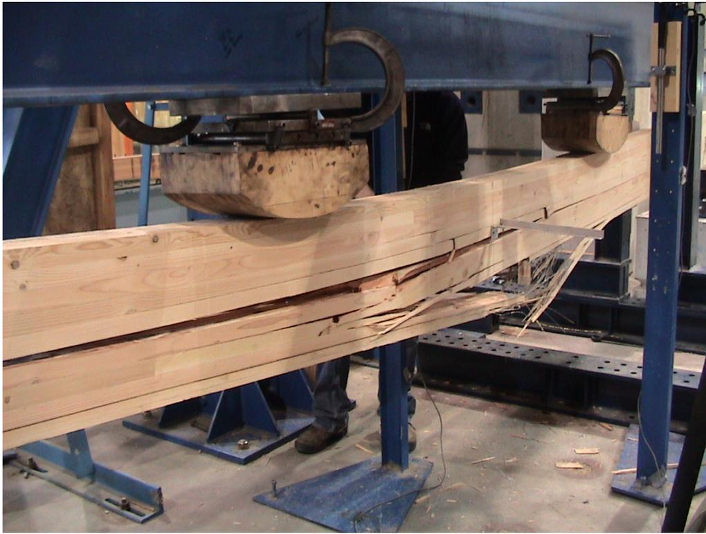
**Figure 10:** Hardwire Reinforced Beam R-3 Tension Failure
