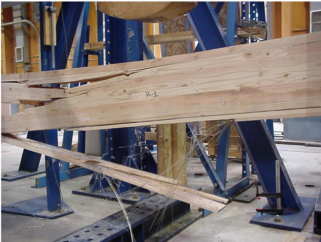
**Figure 7:** Hardwire Reinforced Beam R-1 Tension Failure
