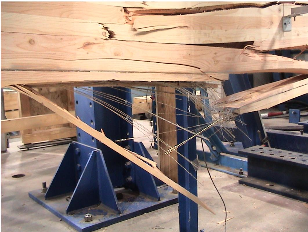
**Figure 9:** Hardwire Reinforced Beam R-2: Close-up of Tension Failure
