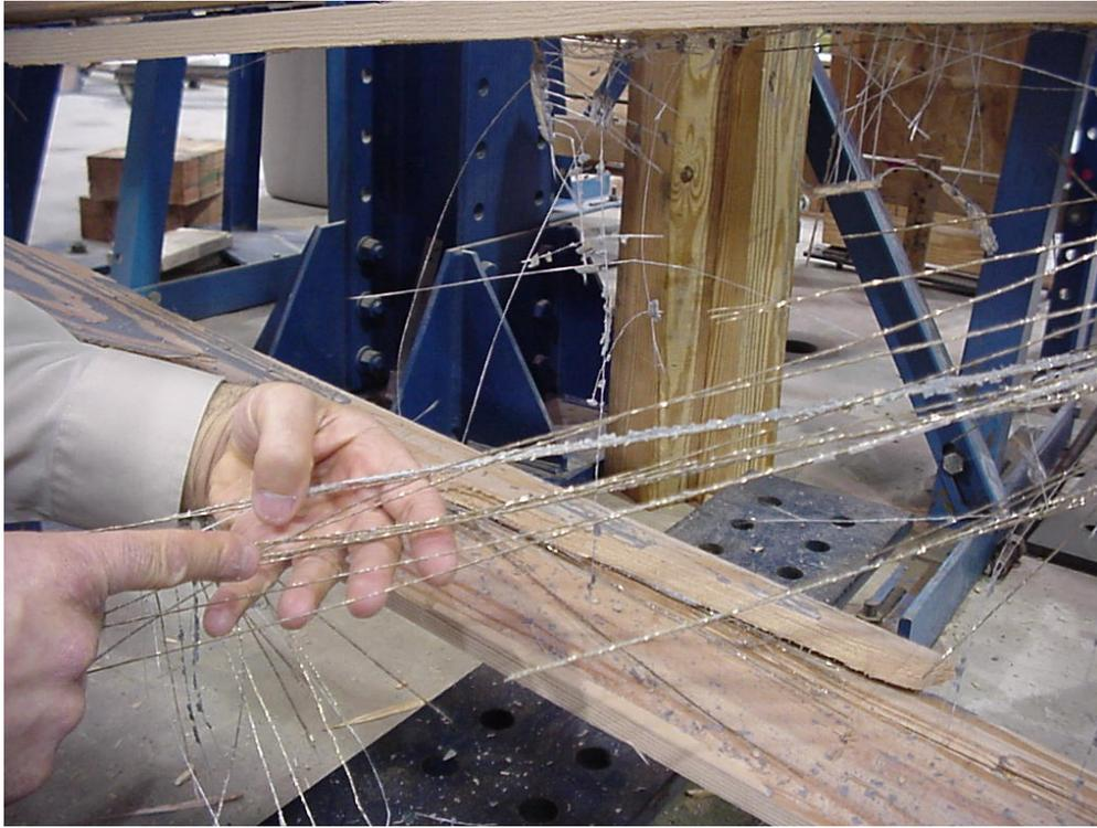
**Figure 4:** Typical condition of steel wires after beam failure for R-1, R-2, & R-3
