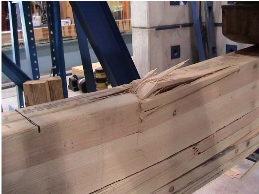
**Figure 5:** Compression failure of beam R-4
