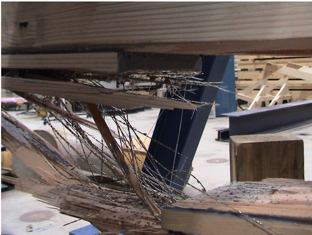
**Figure 11:** Hardwire Reinforced Beam R-3 – Close-up of Tension Failure
