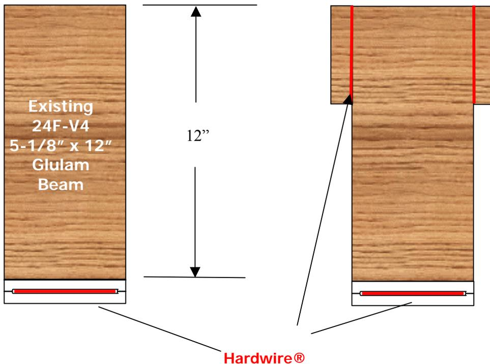
**Figure 1** Beam Section Geometry
