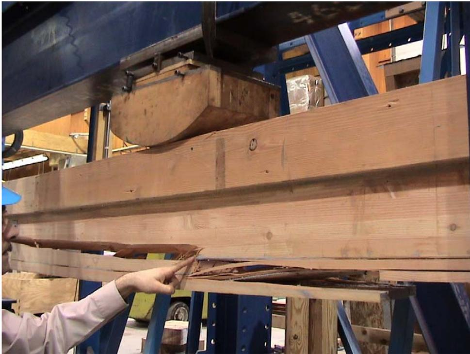
**Figure 14:** R-5 secondary tension failure in the bottom wood lamination of the original glulam. This was accompanied by a horizontal shear failure between the steel reinforcement and the wood directly above it from the load head to the right beam support (See Figure 15)
