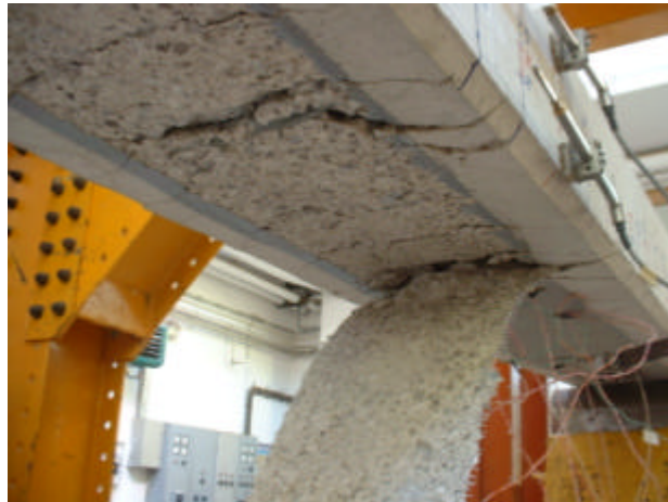
Figure 11: Bottom View of Failure of B-1 Beam
