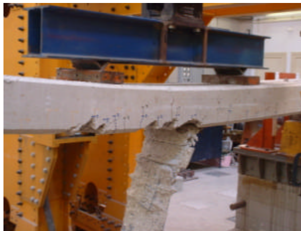
Figure 9: Lateral View of Failure of A-2 Beam
