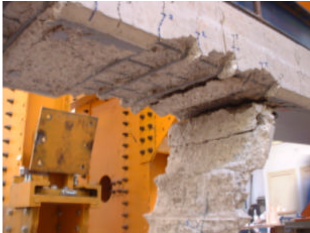
Figure 10: Bottom View of Failure of A-2 Beam
