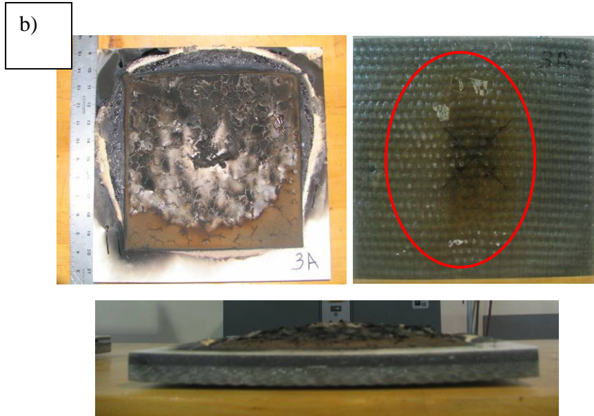
Figure 6. a) Panel 3-A burn through progression (5 minute interval). b) Panel 3-A back face and fire side after burn through testing
